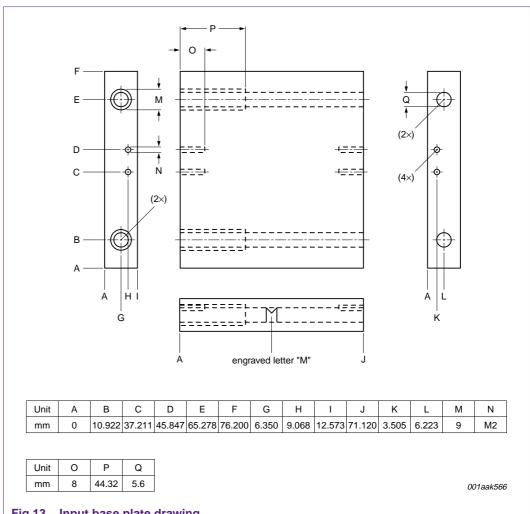
Fig 13. Input base plate drawing
